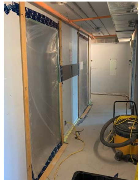
Guarded air tightness testing in progress
